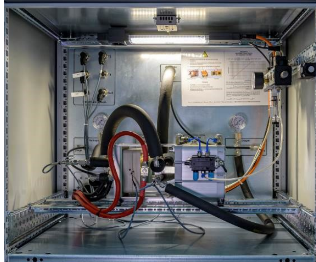
Figure 3: Complete setup of DILICO CURR TEMP in the DILICO HCTS-50 test bench from DILICO engineering GmbH.
